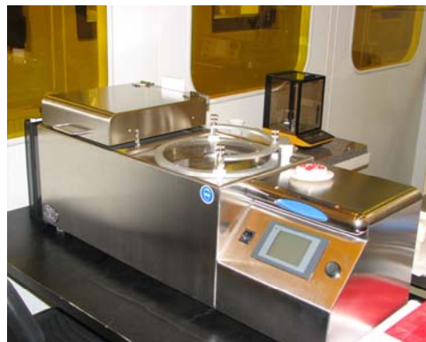
Figure 3 Brewer Science Cee Model 200 Spray Developer for automatic and programmable developing of exposed photoresist
