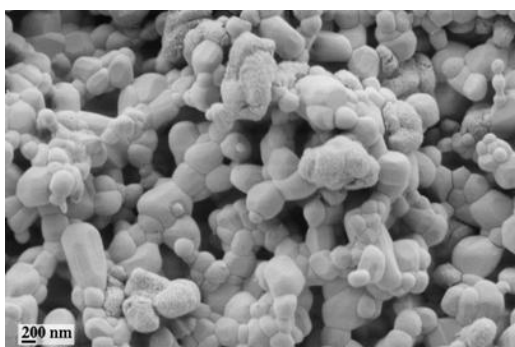
Figure 1 SEM image of HAP powder
