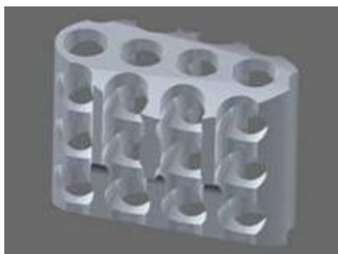
Figure 4 Porous body implant realized by rapid prototyping.
