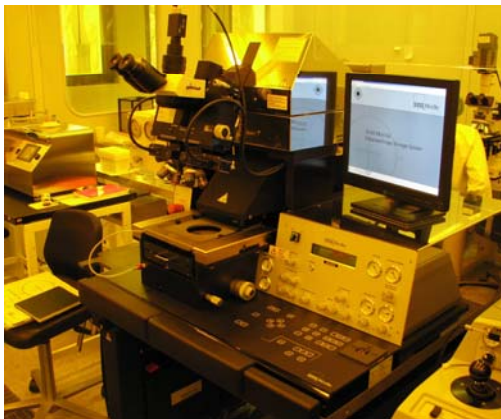
Figure 1 SÜSS MicroTec MA 6 Manual Mask aligner with nanoimprint toolset
