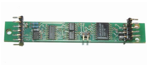
Figure 4 Mini front-end electronics that operates the Fluxset sensor
