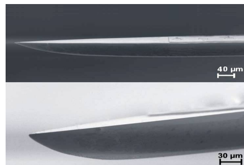
Figure 2 Scanning Electron Micrograph of the completed silicon probe reveals the tip shaped like the bow of a boat and three out of 24 of the Pt recording sites
