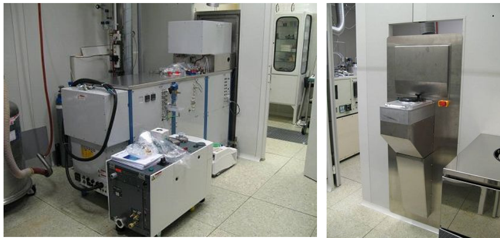
Figure 1 Oxford Instruments Plasmalab 100 DRIE system installed in the clean room
