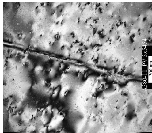
Figure 2 Example of Si grains with dislocation density as high as 8 \cdot 10^9 \text{ cm}^{-2} Plan-view TEM sample
