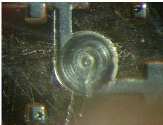
Figure 2 Photograph of the rotating micro-turbine. Here you can see the turbine in action: http://iba.atomki.hu/video/
