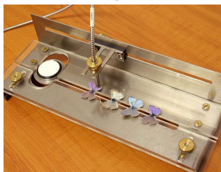
Figure 1 (Color on-line) Photo of installed spectroboard. In the left side there is the Avantes white reference standard. The butterflies are from museum collections, mounted on pins.
