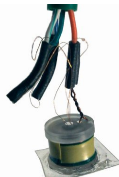
Figure 5 Manufacturing the industrial prototype of the Fluxset probe (Ø 10 mm)
