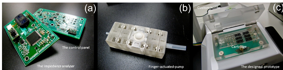
Figure 2. Prototype of the nanopore platform: (a): impedance analyser, (b): finger-actuated micropump, (c): the complete system with the biosensor cartridge.
