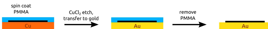
Figure 1. Preparing the gold surface and transfer of CVD graphene onto the gold. In the first step, gold is thermally evaporated onto freshly cleaved mica. A piece of silicon wafer is glued to the top of the gold by epoxy. After the epoxy has cured, the gold can be peeled off the mica surface. The gold surface which was in contact with the mica can then be used as an atomically flat substrate to transfer graphene. The CVD graphene transfer to the gold was done by the standard transfer technique using PMMA.
