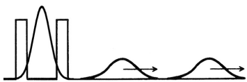
Figure 1a. 1D resonant tunneling. Probability density is shown by a thick line. The quasi localized state in the double barrier region is decaying in distinct impulses.
