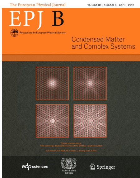
Figure 2a. Spreading of a wave packet on the graphene surface, featured on cover page of EPJ B in 2012. The WP is inserted from an STM tip (not shown) at the middle. Note the anisotropic spreading due to the anisotropic dispersion relation of graphene.
