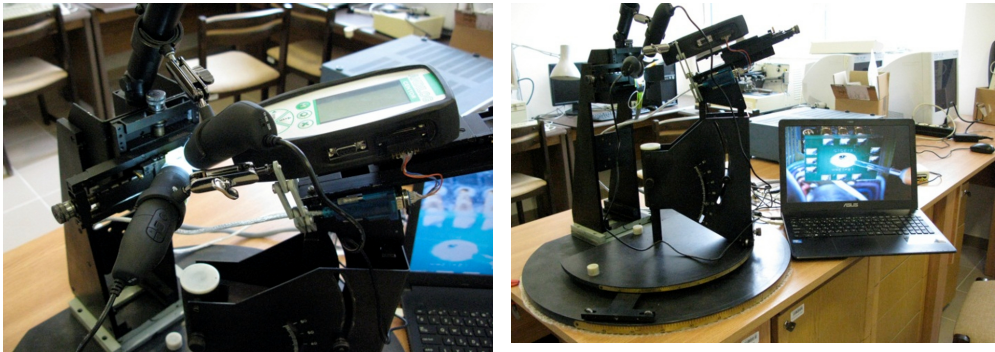
Figure 6. Setup for testing 3D micro-force sensor chip by an accurate force-vector load. Close-up view of the chip and the needle of the calibration force sensor are seen on the monitor of the system control PC.
