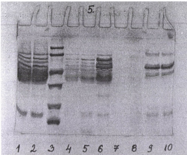
Fig. 2. SDS-PAGE of prolamins of different wheat products. Lane 1: Gluten; Lane 2: Gluten; Lane 3: LMW standard; Lane 4: Wheat germ; Lane 5: Wheat bran; Lane 6: Wheat flake; Lane 7: Wheat starch; Lane 8: Puffed wheat; Lane 9: Rye, Lane 10: Rye
