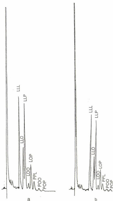
Fig. 5. HPLC of TAG of cottonseed oil (a) before and (b) after 20 min of lipolysis at 55 °C and pH 8.5. LLL: trilinoleoyl-glycerol, LLO: dilinoleoyl-oleoyl-glycerol, LLP: dilinoleoyl-palmitoyl-glycerol, LOO: linoleoyl-dioleoyl-glycerol, LOP: linoleoyl-oleoyl-palmitoyl-glycerol, PPL: dipalmitoyl-linoleoyl-glycerol
