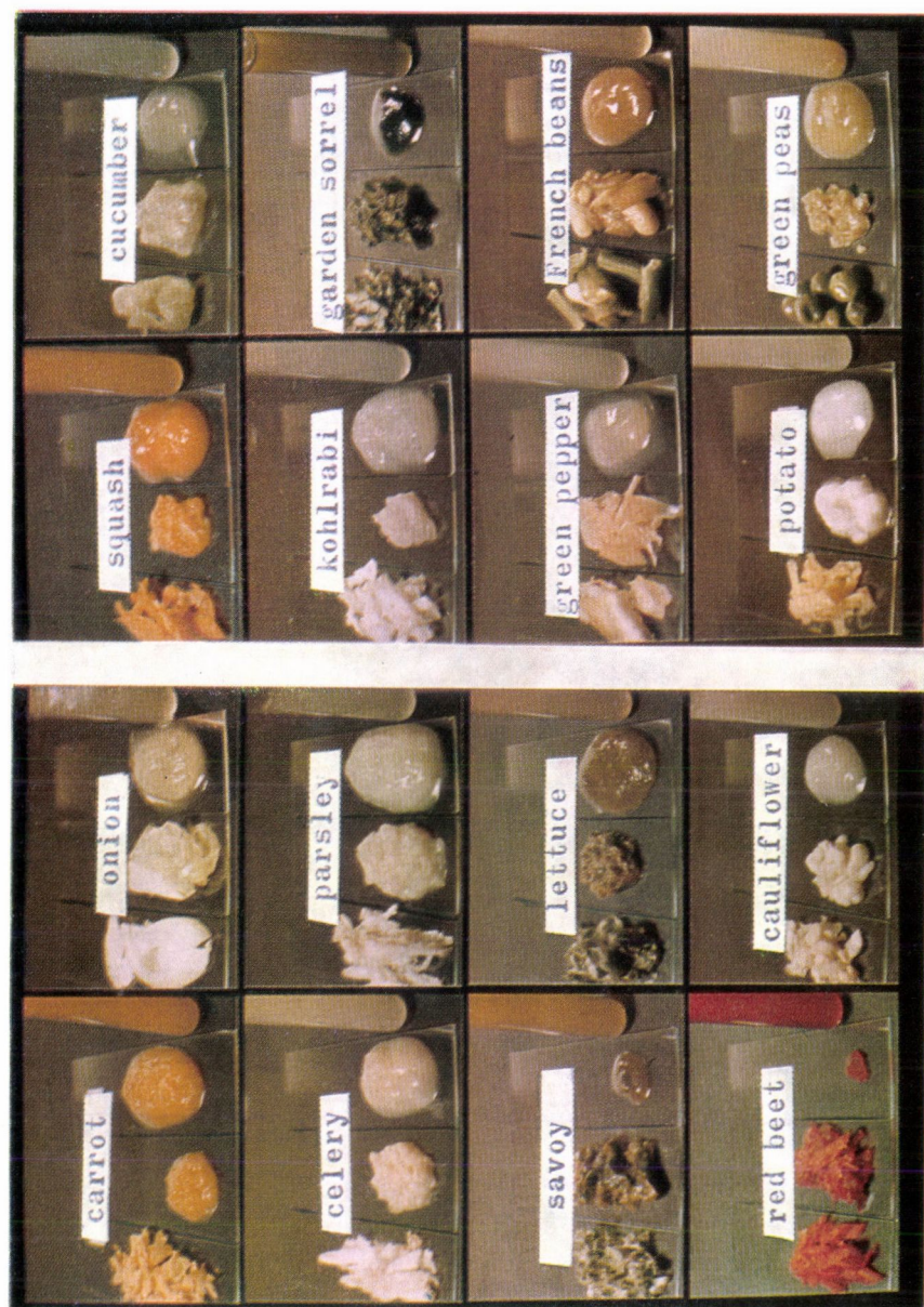
Figs. 5 and 6. Fractions of enzymatically disintegrated vegetable tissues. First slides (from the left): untreated tissues prepared for enzymatic maceration, 2nd and 3rd slides: tissue residues after maceration retained on the 1.0 mm and 0.25 mm screens; test tube: filtrate, containing single cells and cell agglomerates. (Endo-PG: 0.5%; incubation: 3 h at 50 °C)
