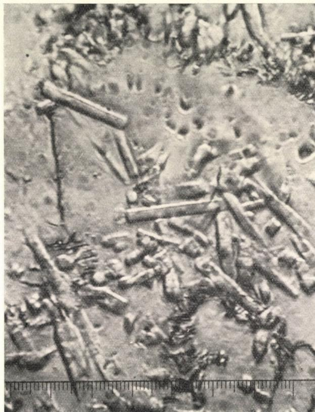
Fig. 6. Polished slide of Grossalmerode potter's clay with large mullite crystals embedded in the glass
