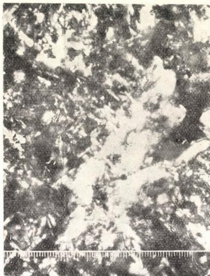
Fig. 3. Polished slide of a glass melting pot made of Grossalmerode clay after 170 hours use in the plant
