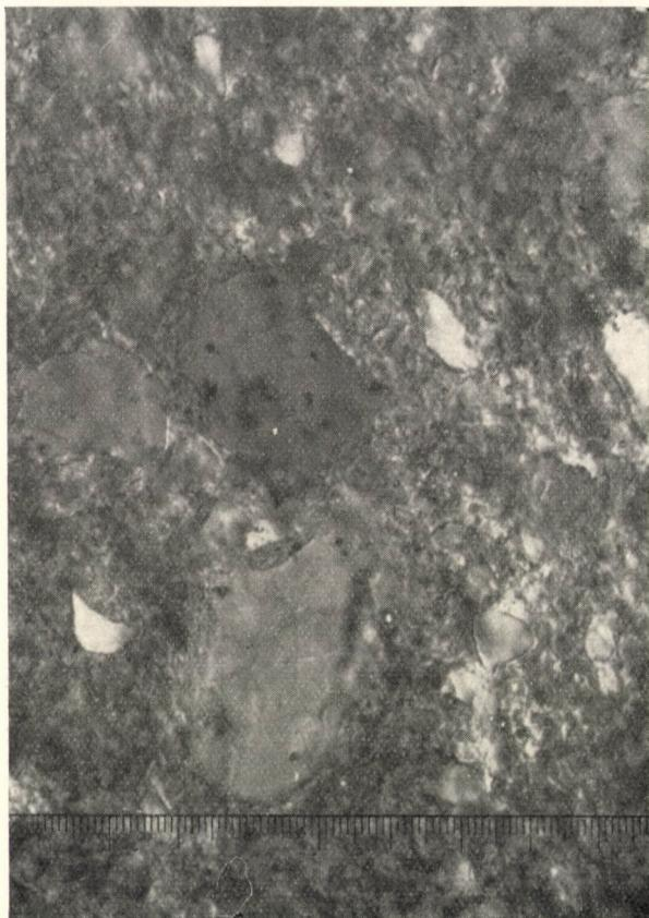
Fig. 2. The texture of Grossalmerode clay after heat treatment at 1400 °C for 6 hours. 800 × magnification in polarized light
