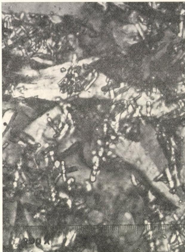
Fig. 5. Polished slide of a glass melting pot made of Grossalmerode clay after 1700 hours use in the plant. The tridymite twin crystals are clearly visible. 800  $\times$  magnification
