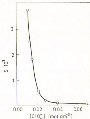
Fig. 5. Solubility of \text{M}(\text{ClO}_4)_3 under the effect of \text{NaClO}_4 in aqueous medium ( t = 25^\circ\text{C} , I = 1 \text{ mol dm}^{-3} , adjusted with \text{NaF} ). Symbols denote experimental results, solid line: solubility curve calculated from the solubility product K_{0,\text{ClO}_4} = 5.43 \times 10^{-9}
