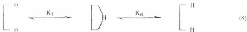
Fig. 3. Protonation equilibria of molecules containing two groups in the case of hydrogen bond formation
