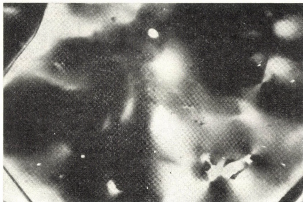
Fig. 10. Polarization micrograph of a poly(phenyl p -acryloiloxy benzoate)film
