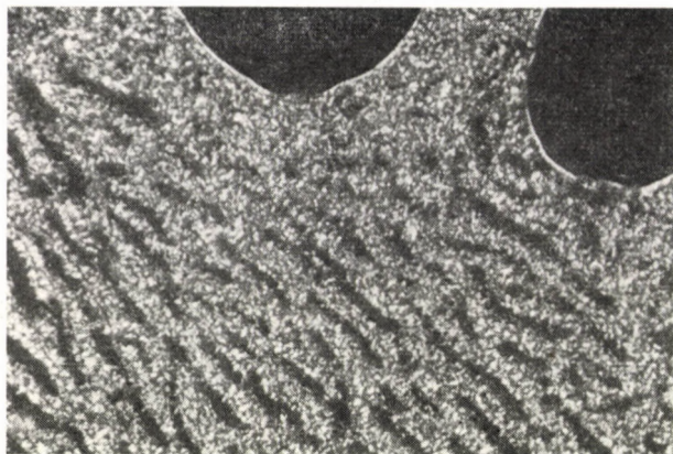
Fig. 6. Polarization micrograph of poly(cholesteryl vinyl succinate)
