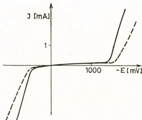
Fig. 3. Polarization curve of the iron electrode in a 0.05 N sodium acetate solution containing 20 per cent acetone
