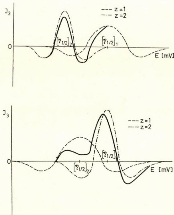
Fig. 5. Vectorial summation of third harmonic A.C. polarograms (explanation in the text)
