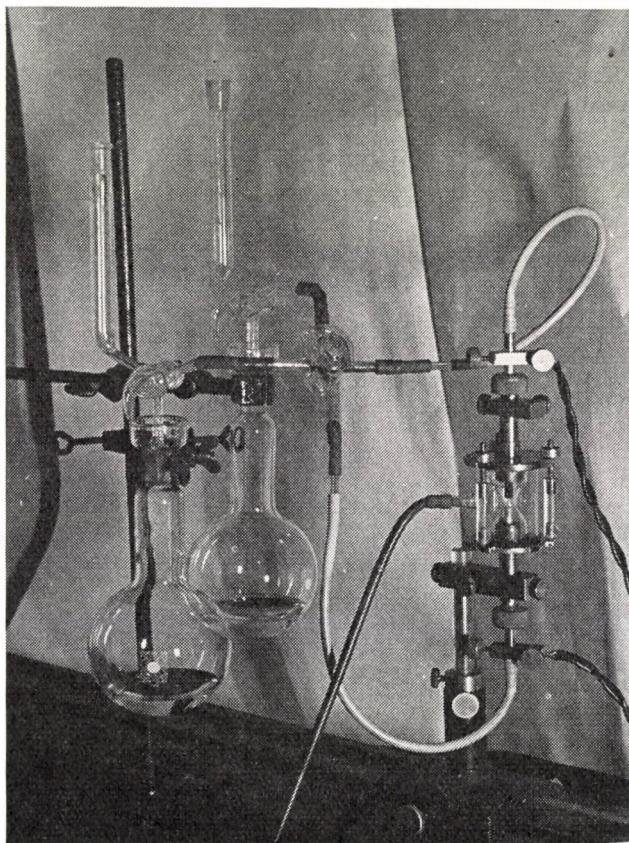
Fig. 4. Gas cell with reaction flasks assembled
