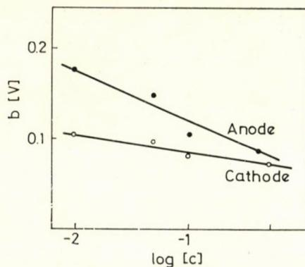
Fig. 6.  $b$  constants of Tafel's equation as plotted vs. the sodium acetate concentration
