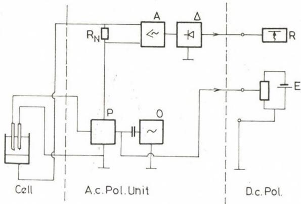
Fig. 6. Block diagram of the A.C. polarographic instruments
