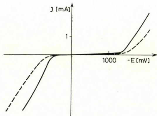
Fig. 2. Polarization curve of the iron electrode in a 0.01 N sodium acetate solution containing 10 per cent acetone
