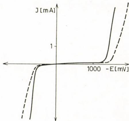
Fig. 4. Polarization curve of the iron electrode in a 0.1 N sodium acetate solution containing 10 per cent acetone
