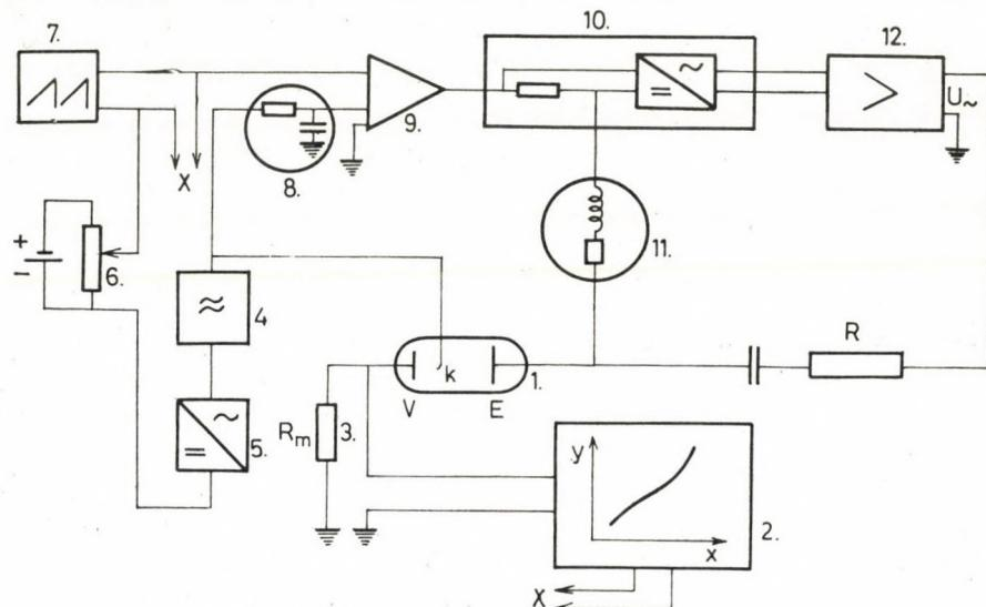
Fig. 1. Block diagram of the equipment. 1. Cell; 2. X—Y recorder; 3. Measuring resistance; 4. Wave analyser; 5. Demodulator; 6. Potentiometer; 7. Kipp generator; 8. Filter circuit; 9. Potentiostat; 10. Modulator; 11. Filter circuit; 12. Amplifier
