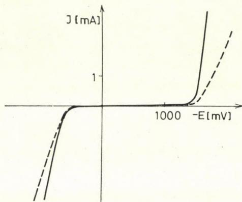
**Fig. 5.** Polarization curve of the iron electrode in a 0.5 N sodium acetate solution containing 10 per cent acetone
