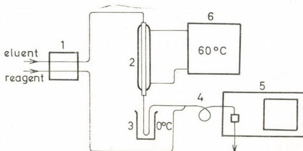
Fig. 2. Chromatographic apparatus for the separation of antipyrine derivatives. 1 peristaltic pump; 2 ion exchange column with heating jacket; 3 cooler; 4 mixing coil; 5 photometer; 6 thermostat
