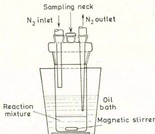
Fig. 8. Apparatus designed for the kinetic measurements
