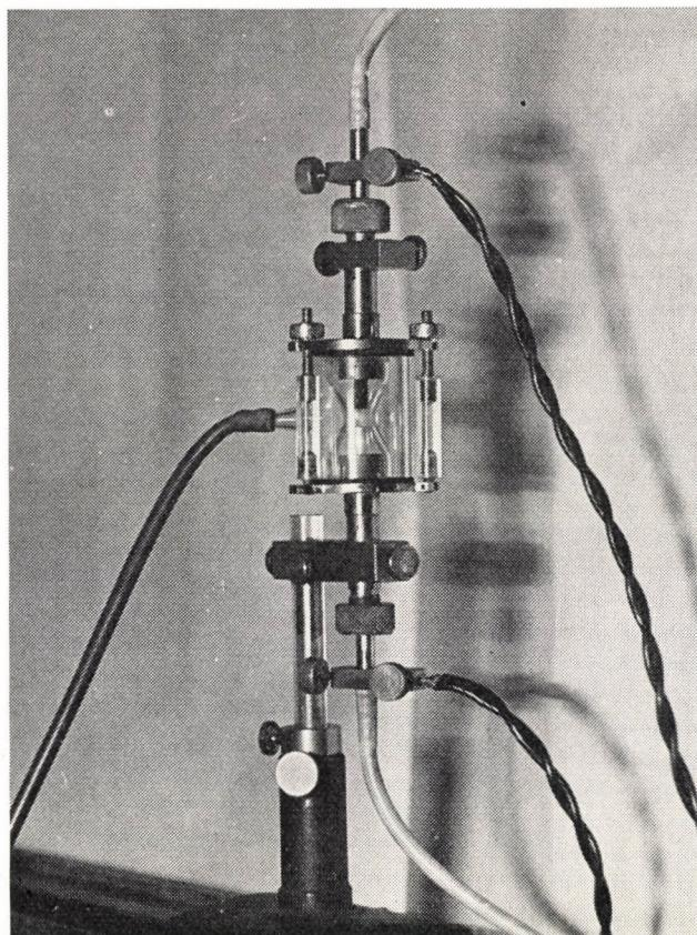
Fig. 1. Electrode stand with gas cell
