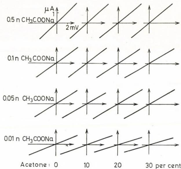
Fig. 7. Corrosion current density data as a function of sodium acetate and acetone concentrations, respectively
