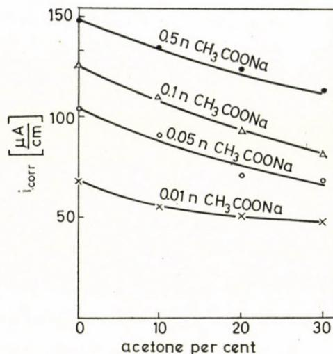
Fig. 8. Corrosion current density data as a function of the acetone concentration
