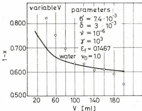
Fig. 10. Gas fraction of foam vs. volume of liquid. Variable  $V$
