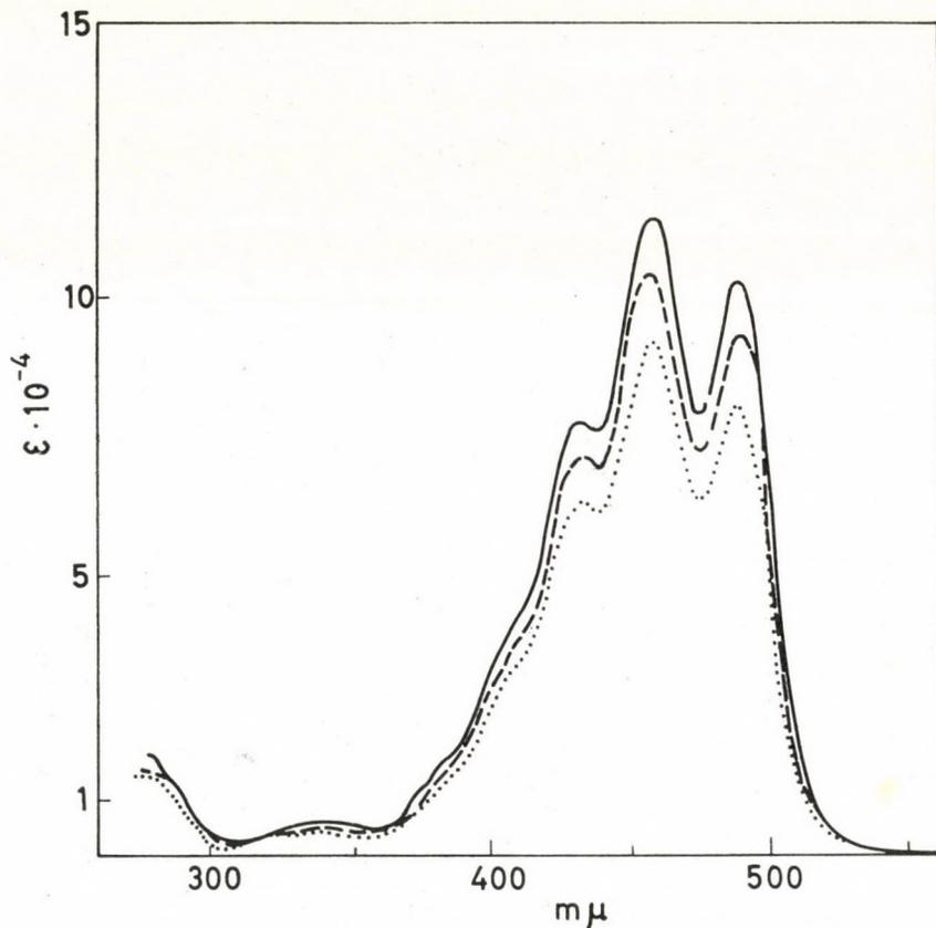
Fig. 1. Molar extinction curves of isozeaxanthin monoepoxides in benzene. Isozeaxanthin monoepoxide A — ( $\lambda_{\max}$  488, 459, and 339  $m\mu$ ); isozeaxanthin monoepoxide B - - - ( $\lambda_{\max}$  489, 459 and 339  $m\mu$ ); isozeaxanthin monoepoxide C . . . ( $\lambda_{\max}$  489, 458 and 339  $m\mu$ )
