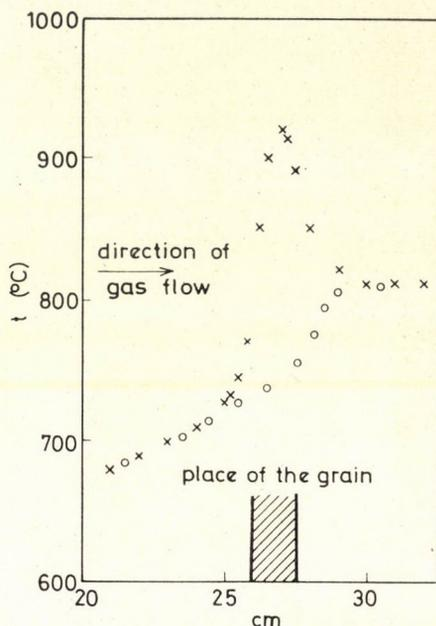
Fig. 1b. Temperature distribution along the reactor. Symbols:  $\times$  measured with the thermometer passing through the grain;  $\circ$  measured with the thermometer alongside the grain
