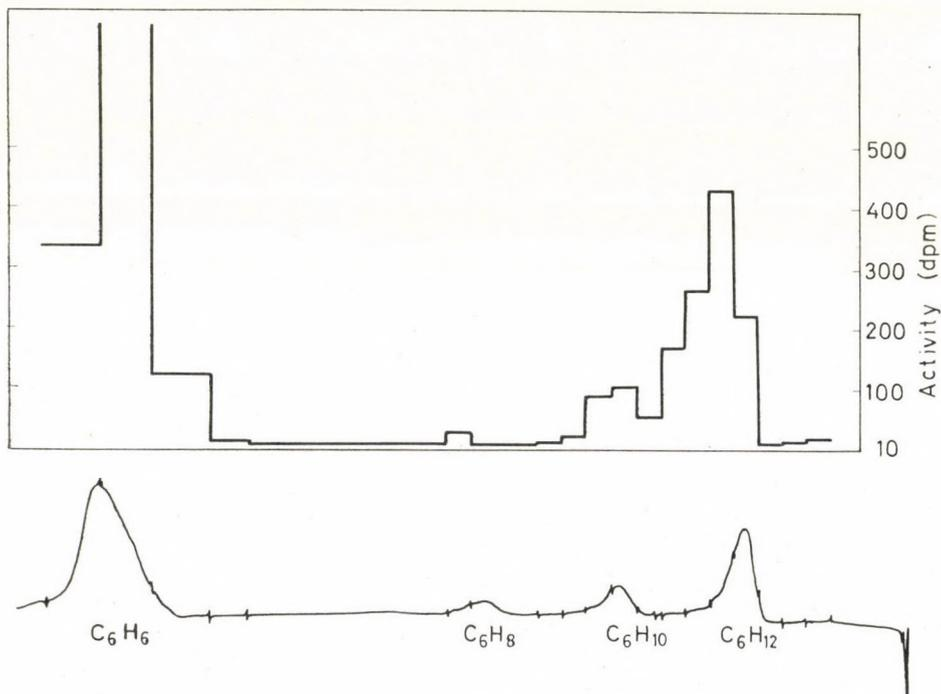
Fig. 1. Typical chromatogram of a hydrogenation run (mixture of benzene- $^{14}\text{C}$  and cyclohexadiene) and the absolute radioactivities of narrow fractions. (The places of fraction changes are shown by small deflections on the chromatogram.) Catalyst: 1.7 mg of Pt;  $t = 190^\circ\text{C}$ ;  $3\ \mu\text{l}$  of 1 : 1 mixture,  $V(\text{H}_2) = 60\ \text{ml/min}$ . Radioactivity peaks are corrected for the background
