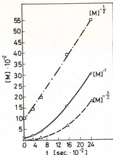
Fig. 1. Kinetical course of the polymerization of acrylamide.  $[M_0] = 2.816$  mole/l;  $[K_2S_2O_8] = 1.5 \times 10^{-2}$  mole/l; [ascorbic acid] =  $1 \times 10^{-2}$  mole/l; pH = 4.5; temp. =  $25^\circ C$
