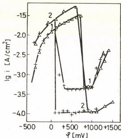
Fig. 2. Potentiostatic polarization curves recorded by sweeping the potential in positive ( $\Delta$ ) and (+) opposite directions in a 0.5 M  $\text{CH}_3\text{COONa}$  solution. Solvents: 1 — 90%  $\text{CH}_3\text{COOH}$  + 10%  $\text{H}_2\text{O}$ , 2 — 50%  $\text{CH}_3\text{COOH}$  + 50%  $\text{H}_2\text{O}$
