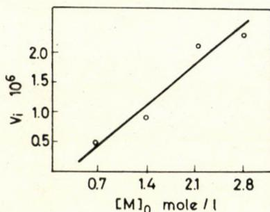
Fig. 7. Change of the rate of initiation with the monomer concentration.  $[I] = 6.16 \times 10^{-3}$  mole/l; pH = 4.5; temp. = 25 °C
