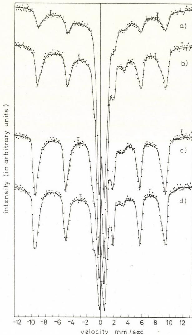
Fig. 4. Effect of preheating at 60 °C on the Mössbauer spectrum measured at 77 °K in a solution with pH = 2.20. a) without preheating. Time of preheating b) 45 min; c) 2h; d) spectrum c measured after 20 days
