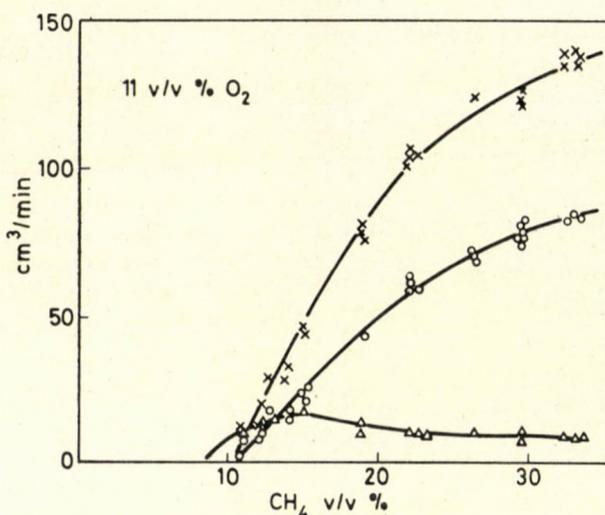
Fig. 10. Rate of formation of the products as a function of methane concentration. Symbols: × hydrogen; ○ carbon monoxide; △ carbon dioxide
