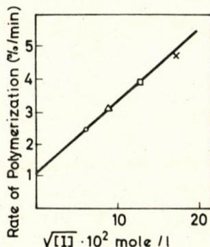
Fig. 2. Initial rate of polymerization of acrylamide as a function of the square root of the concentration of the initiator system.  $[M_0] = 1.408$  mole/l; pH = 4.5; temp. = 25 °C
