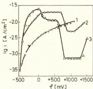
Fig. 3. Potentiostatic polarization curves recorded in a 0.15 M sodium acetate solution. Solvents: 1 — anhydrous acetic acid, 2 — 96.7% CH<sub>3</sub>COOH + 3.3% H<sub>2</sub>O, 3 — 90% CH<sub>3</sub>COOH + 10% H<sub>2</sub>O
