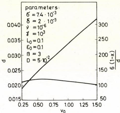
Fig. 4. Average bubble diameter and specific surface of foam calculated from Eqs (37) and (13) vs. linear gas rate
