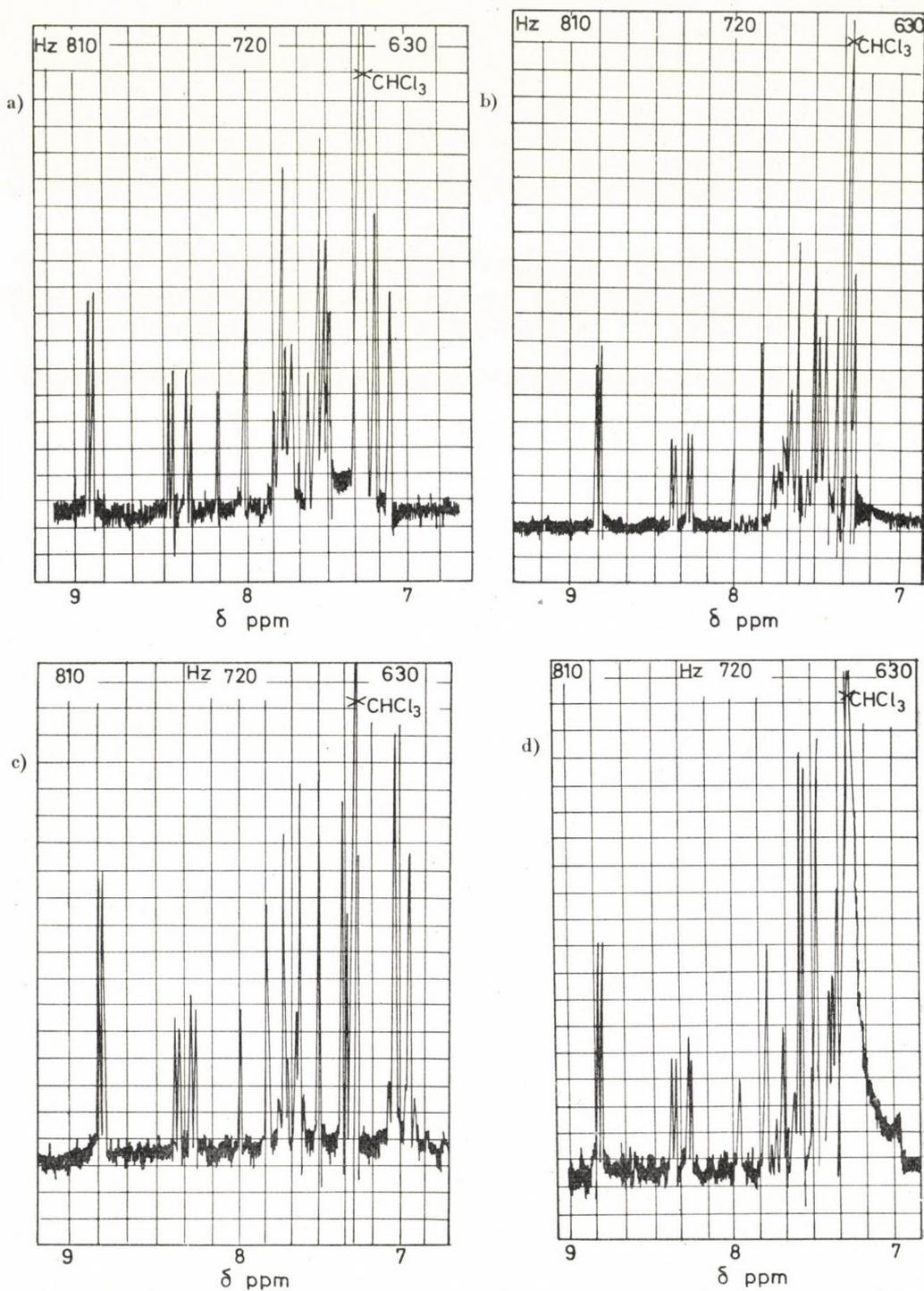
Fig. 4. 90 MHz proton resonance spectra of compounds **Ia**–**Id** in deuteriochloroform solution in the range of  $\delta = 6.5$ – $9.0$  ppm. a) 5'-Nitro-2'-hydroxychalcone (**Ia**). b) 3'-Nitro-4'-hydroxychalcone (**Ib**). c) 3'-Nitro-4'-hydroxy-4-methoxychalcone (**Ic**). d) 3'-Nitro-4'-hydroxy-4-chlorochochalcone (**Id**)
