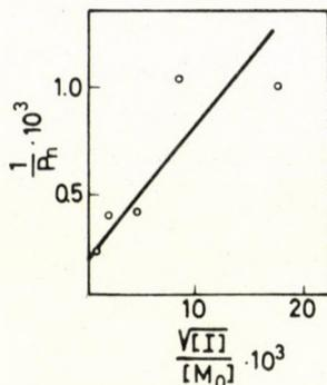
Fig. 5. Reciprocal of the number average degree of polymerization  $\left(\frac{1}{\bar{P}_n}\right)$  against  $\frac{\sqrt{[I]}}{[M_0]}$
