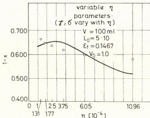
Fig. 11. Gas fraction of foam vs. dynamic viscosity. Variable  $\eta$
