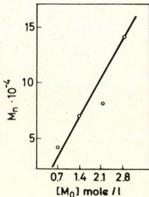
Fig. 3. The number average molecular weight of polyacrylamide ( $M_n$ ) plotted against the initial monomer concentration  $[M_0]$ .  $[I] = 6.16 \times 10^{-3}$  mole/l; pH = 4.5; temp. = 25 °C
