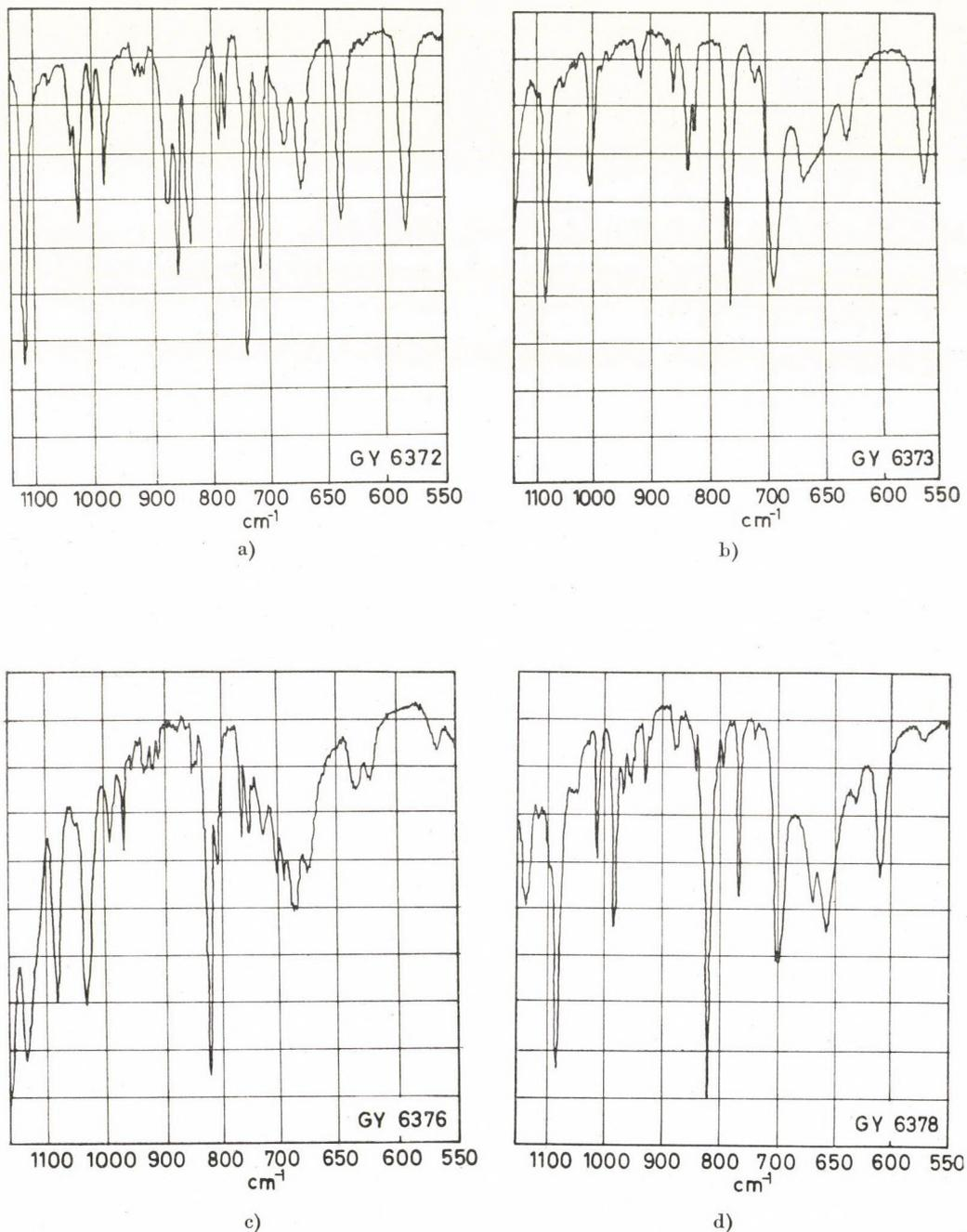
Fig. 1. IR spectra of compounds **Ia**–**Id** in the range of 1100–600 cm<sup>-1</sup> in KBr pellets (2-fold scale expansion is twice below 700 cm<sup>-1</sup>). a) 5'-Nitro-2'-hydroxy-chalcone (**Ia**); b) 3'-Nitro-4'-hydroxy-chalcone (**Ib**); c) 3'-Nitro-4'-hydroxy-4-methoxychalcone (**Ic**); d) 3'-Nitro-4'-hydroxy-4-chlorochalcone (**Id**)
