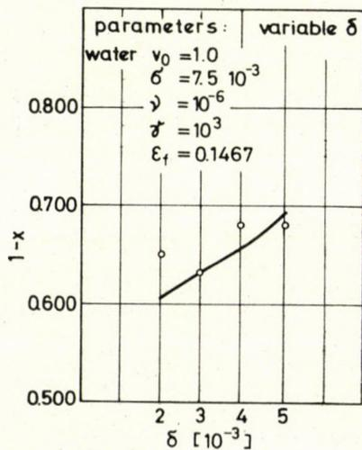
Fig. 7. Gas fraction of foam vs. opening diameter. Variable  $\delta$
