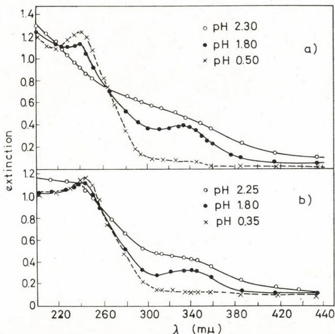
Fig. 1. Variation of spectrophotometric curves with the pH of solutions a) in 3 M  $\text{NaClO}_4$ , b)  $\ll 3 \text{ M NaClO}_4$  in ferric perchlorate solution
