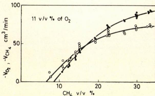
Fig. 9. Variation of the conversion rate of methane and oxygen as a function of the concentration of methane. Symbols: ● methane; ○ oxygen
