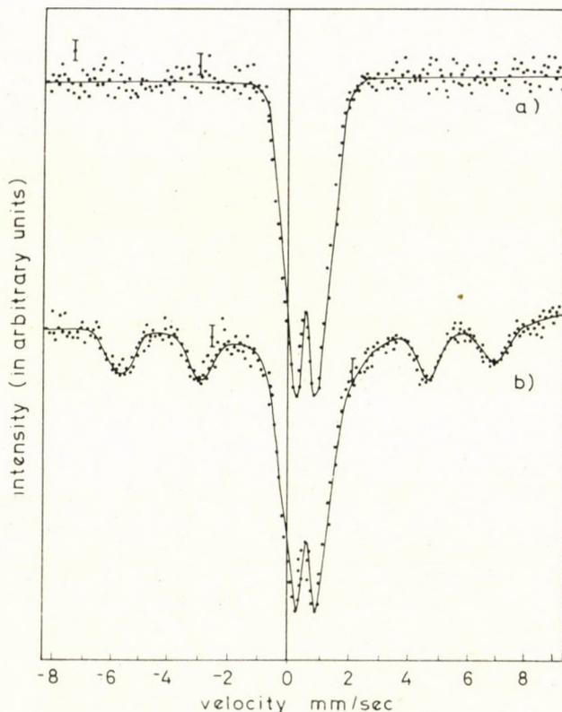
Fig. 5. Mössbauer spectrum of a solution of pH = 2.35, measured at 77 °K a) immediately after pH adjustment; b) after standing for 26 days
