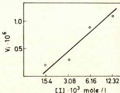
Fig. 8. Change of the rate of initiation with the concentration of the redox system.  $[M_0] = 1.408$  mole/l; pH = 4.5; temp. = 25 °C
