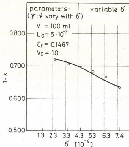
Fig. 9. Gas fraction of foam vs. surface tension. Variable  $\sigma$
