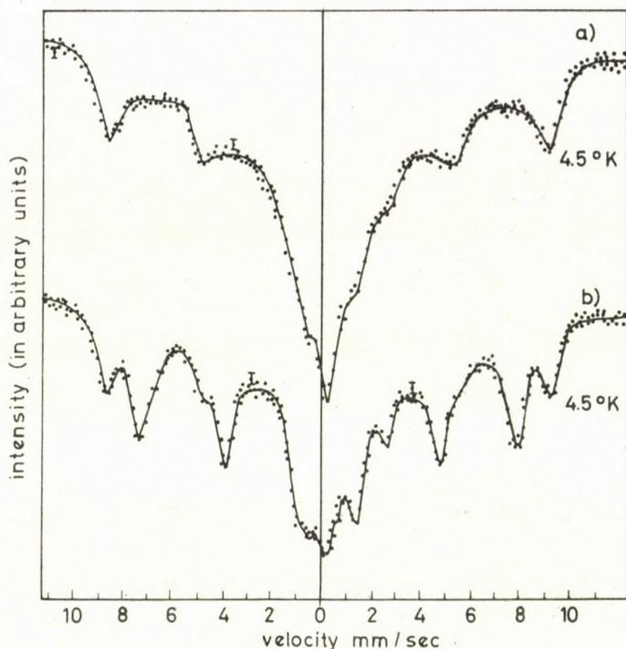
Fig. 3. Mössbauer spectra of frozen solutions with pH = 1.40. a) without preheating, b) solution preheated at 60 °C for 45 min before freezing
