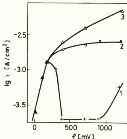
Fig. 6. Effect of speed of rotation of the electrode on the shape of the potentiostatic curve recorded on 0.2 M HClO<sub>4</sub> solution prepared with anhydrous acetic acid. The rpm of the rotating disc electrode: 1 -  $f = 0 \text{ min}^{-1}$ , 2 -  $f = 230 \text{ min}^{-1}$ , 3 -  $f = 1320 \text{ min}^{-1}$
