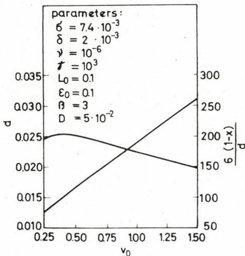
Fig. 5. Average bubble diameter and specific surface of foam calculated from Eqs (37) and (14) vs. linear gas rate. Variable  $v_0$
