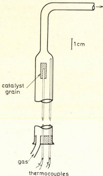
Fig. 1a. Schematic diagram of the single-grain reactor
