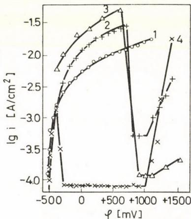
Fig. 1. Potentiostatic polarization curves for iron electrodes immersed into a 0.5 M  $\text{CH}_3\text{COONa}$  solution. Composition of the solvent: 1 — anhydrous acetic acid, 2 — 90% acetic acid + 10% water, 3 — 50% acetic acid + 50% water, 4 — 100% water
