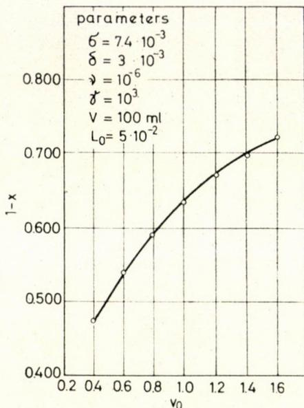
Fig. 6. Gas fraction of foam vs. linear rate of forced-in gas. Variable  $v_0$
