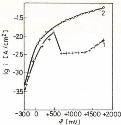
Fig. 5. Potentiostatic polarization curves recorded in a 0.2 M  $\text{NaClO}_4$  solution. Solvents: 1 — anhydrous acetic acid, 2 — 98%  $\text{CH}_3\text{COOH}$  + 2%  $\text{H}_2\text{O}$
