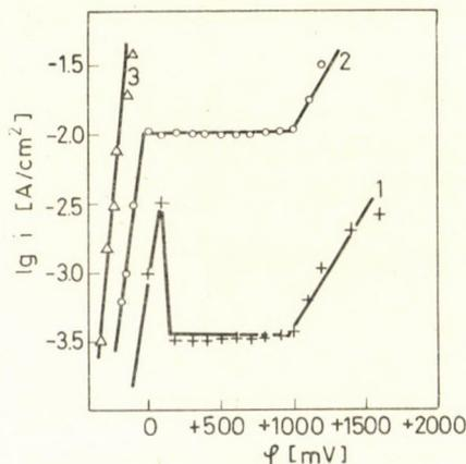
Fig. 4. Potentiostatic polarization curves recorded in a 0.5 M perchloric acid solution. Composition of the solvent: 1 — anhydrous acetic acid, 2 — 98% CH<sub>3</sub>COOH + 2% H<sub>2</sub>O, 3 — 90% CH<sub>3</sub>COOH + 10% H<sub>2</sub>O
