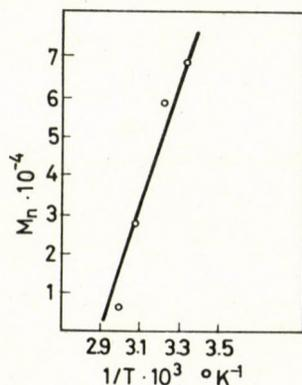
Fig. 6. Effect of temperature on the molecular weight ( $\bar{M}_n$ ).  $[M_0] = 1.408$  mole/l;  $[I] = 6.16 \times 10^{-3}$  mole/l; pH = 4.5
