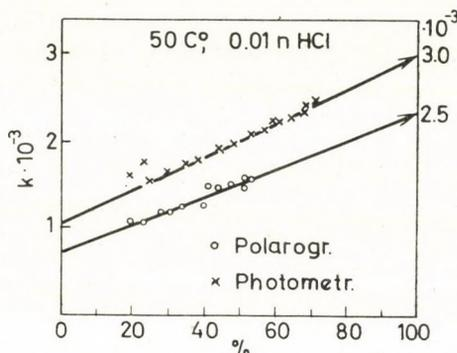
Fig. 2. Increase of the rate constant with the progress of hydrolysis
