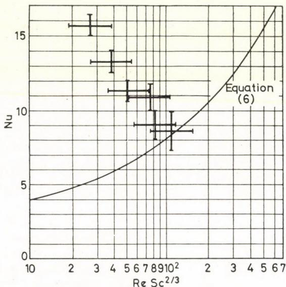
Fig. 1. Graphical representation of the results of component transfer measurements plotted as the relationship of dimensionless parameters
