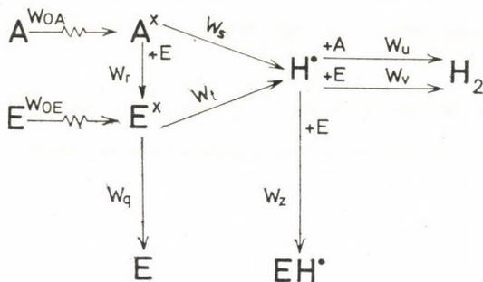
Fig. 17. Proposed hydrogen formation scheme
