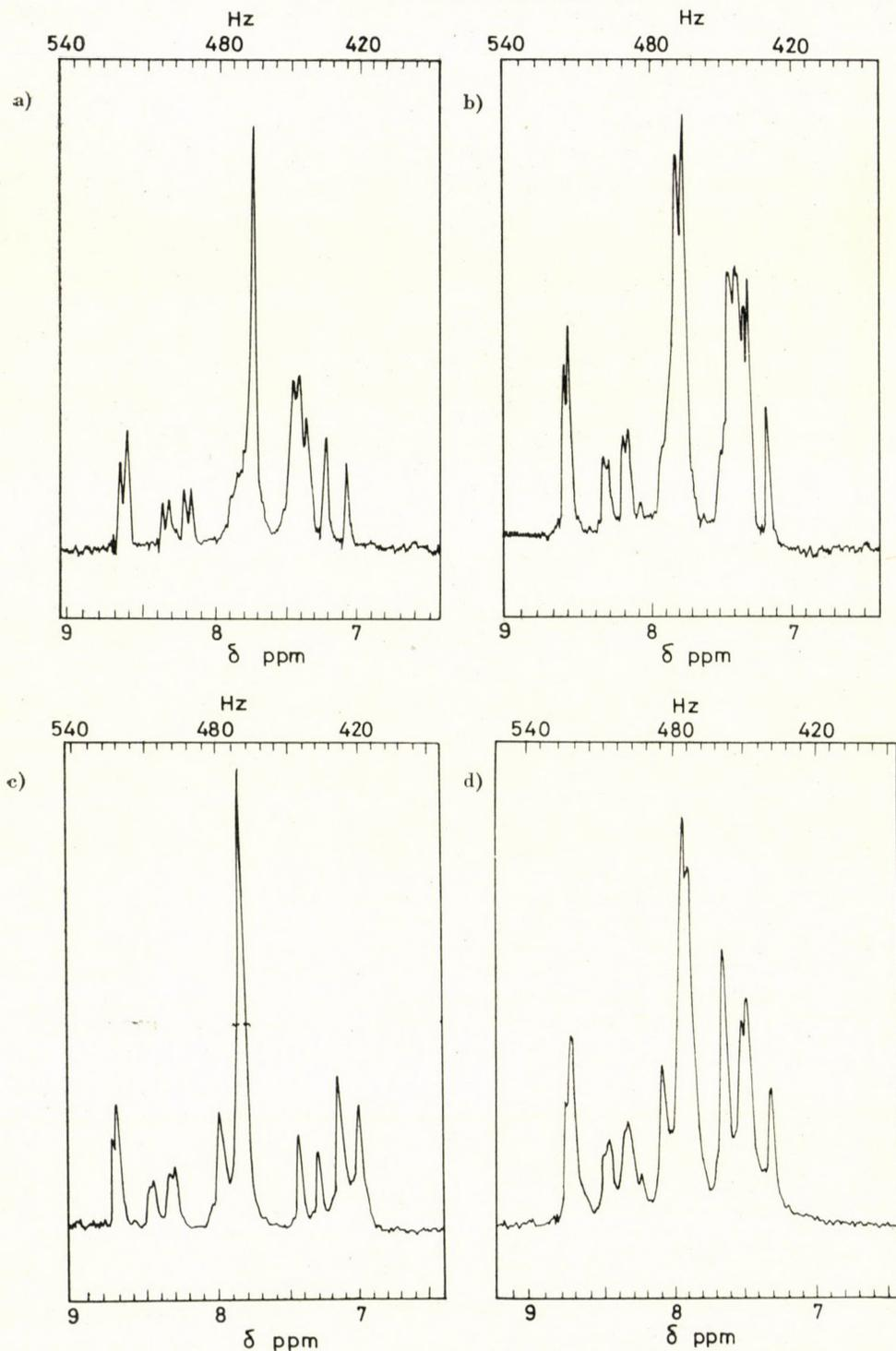
Fig. 3. The 60 MHz proton resonance spectra of compounds **Ia**–**Id** in deuterio-dimethyl sulfide solution in the range of  $\delta = 6.5$ – $9.0$  ppm. a) 5'-Nitro-2'-hydroxy-chalcone (**Ia**); b) 3'-Nitro-4'-hydroxy-chalcone (**Ib**). c) 3'-Nitro-4'-hydroxy-4-methoxychalcone (**Ic**). d) 3'-Nitro-4'-hydroxy-4-chlorochalcone (**Id**)
