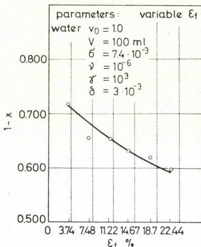
Fig. 8. Gas fraction of foam vs. fraction of openings. Variable  $\epsilon_f$
