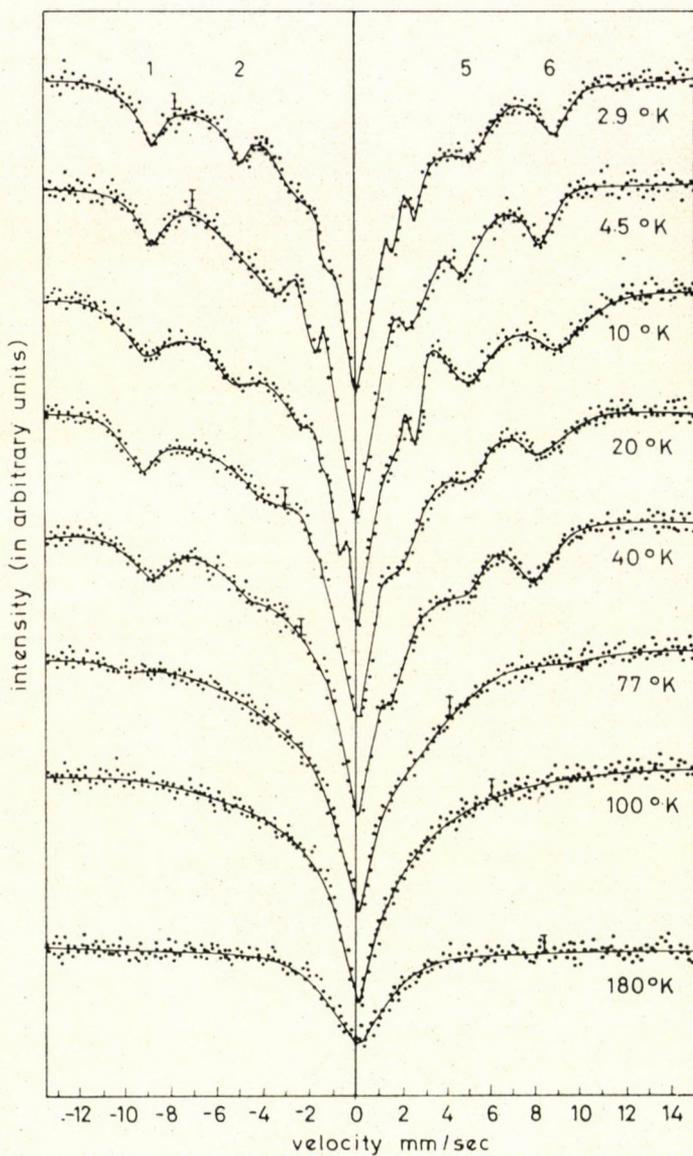
Fig. 2. Variation of Mössbauer spectra with temperature in solutions at different values of the pH. a) pH = 0.40
