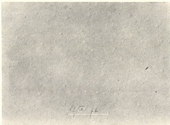
Fig. 6. Surface treated with the etching mixture CPI, continuous oxide layer. Direct magnification, \times 32\,000
