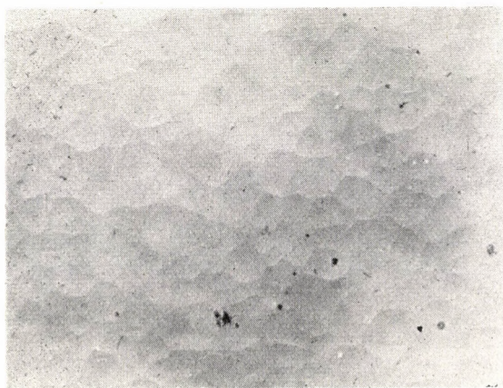
Fig. 17. Surface treated with hydrogen peroxide containing lithium carbonate, at 25 °C for 71 hours. Direct magnification, \times 2000
