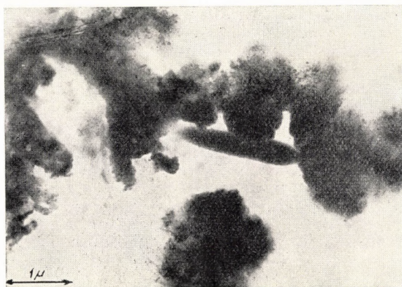
Fig. 4. Electron microscopic photograph of uranium(VI) in NaOH solution [5 mg of U(VI) dissolved in 100 ml of 0.1 N NaOH. The solution was evaporated on a Formvar carrier film, and the photograph taken with an electron microscope of Type Tesla BS 242. Accelerator voltage: 60 kV. Magnification: 5000 \times .]
