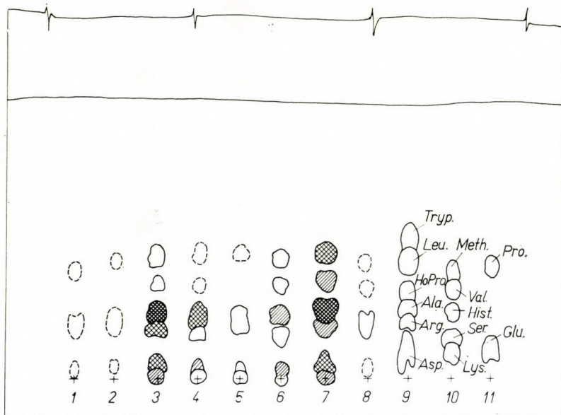
Fig. 9. Thin-layer chromatogram of supernatant of vegetative and resting spore suspensions. 1. Vegetative cells, 0 krad; 2. Vegetative cells, 100 krad; 3. Vegetative cells, 500 krad; 4. Vegetative cells, 70°C, 5 minutes; 5. Resting spores, 0 krad; 6. Resting spores, 500 krad; 7. Resting spores, 1000 krad; 8. Resting spores, 90°C, 100 minutes; 9., 10., 11. Amino acid solutions for comparison
