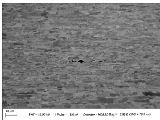
Fig. 3. ECCI image of a specimen stretched by 4% in a section perpendicular to the stretching direction
