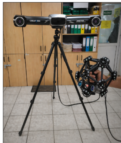
Fig. 1. MetraSCAN 750 Elite scanner.
