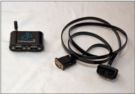
Fig. 1. The CANedge2 device and OBD2 cable.
