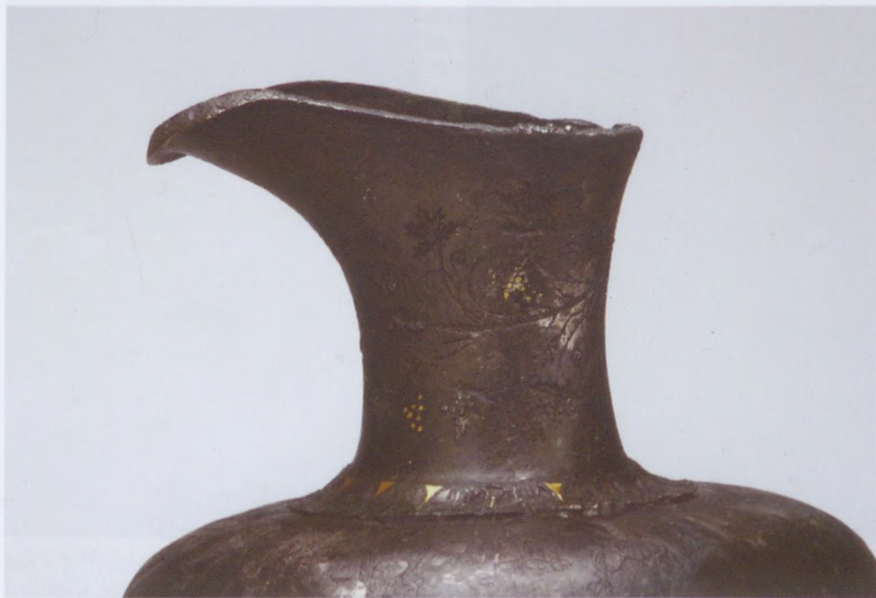
Fig. 20 Detail of the neck with some remains of a gold inlay with wine leaves and grapes motive. Previously prepared wax models might have been used for the less important parts, such as neck and foot. (Courtesy of Hungarian National Museum, photo: András Dabasi)
