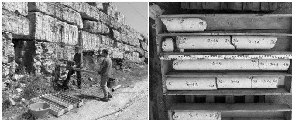
Figure 7. Sampling by Hilti-drilling and core boxes
