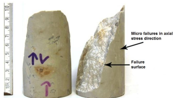
Figure 11. Shear failure PK 1 – Neuburger Bankkalk –
