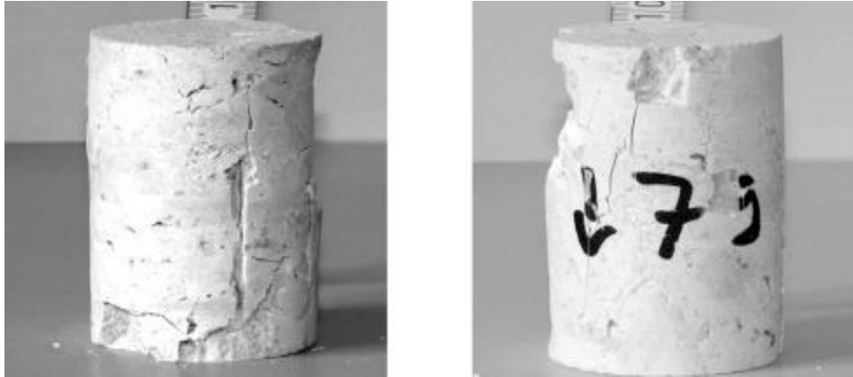
Figure 8. Form of failures after uniaxial loading tests, Kelheimer Kalk B. 3-1-A, PK 79
