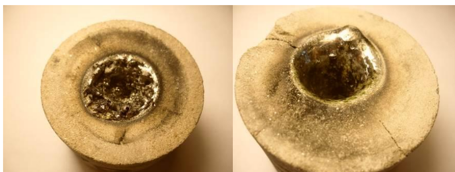
Figure 4. Laser drilled holes with melted smooth and bubble containing surfaces with and without heat shock induced fractures
