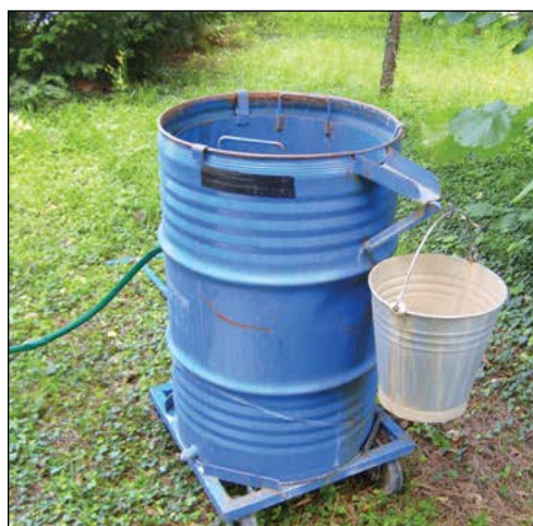
Fig. 4. Flotation equipment and its operating principle. Constructed by Á. Kenéz.
