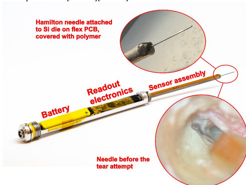
Figure 51. Handheld tissue tester with the sensor assembly before transection of the chorda tympani nerve.
