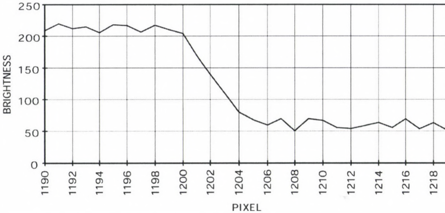
Fig. 6. The dark-bright transition of a CCD image line sensor at the moving edge
