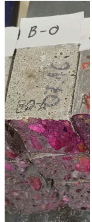
Figure 5: CEM II specimens after the acid test
