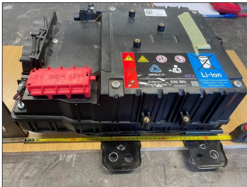
Figure 1 Unassembled Ford Transit battery pack
