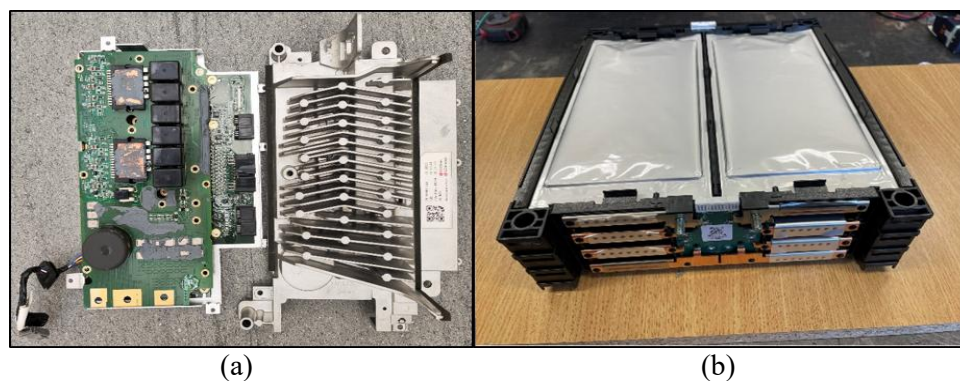
Figure 2 Main units of the hybrid system, (a) inverter and (b) battery pack.
