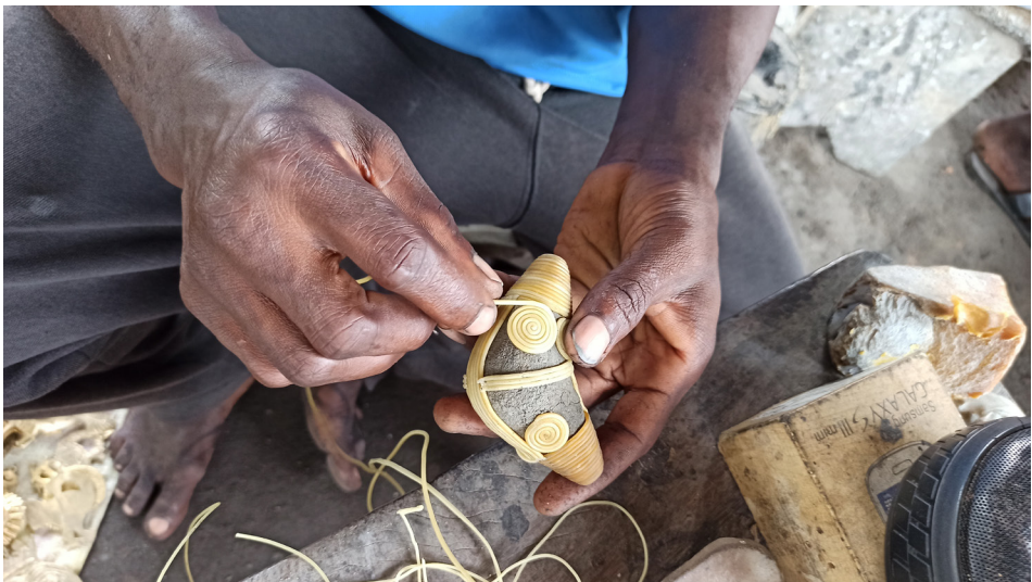
20. The Kumasi region is famous for its brass and bronze production. Using the lost-wax casting process, artisans create beads in various shapes and with different motifs from beeswax wire. Sokoban Krofrom, Kumasi, 1 May 2023
