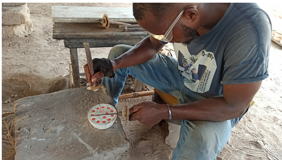
13. Just after firing, each bead is pierced with a homemade pricker and shaped by turning it in the hole of the mold. This operation requires great skill and practice.
