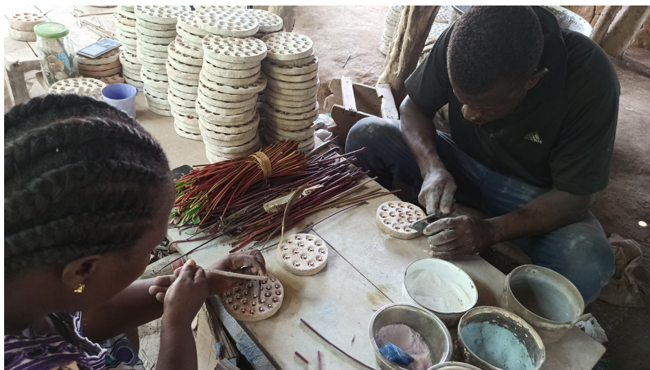
5. Pouring painted powdered glass into the mould with tin funnels, also creating motifs with different colours
