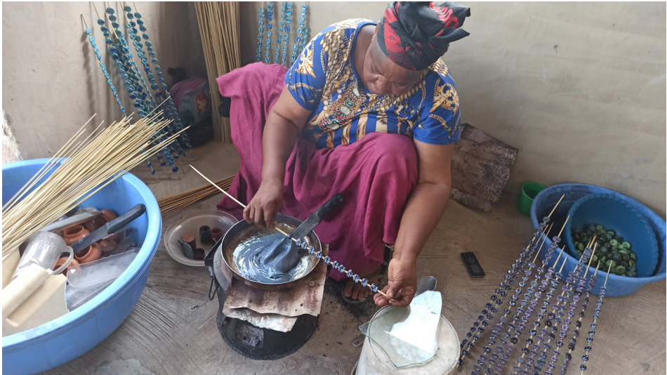
19. Twenty years ago, Mrs. Amina discovered – through a kitchen accident she saw as divine guidance – how to make beads from melted plastic. In a space of less than two square meters, using simple kitchen utensils, she produces thousands of beads in various colours and shapes. Kumasi, 20 May 2023
