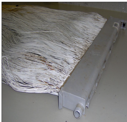
Fig. 13. Membrane technology membrane module element in Karcag [3]
