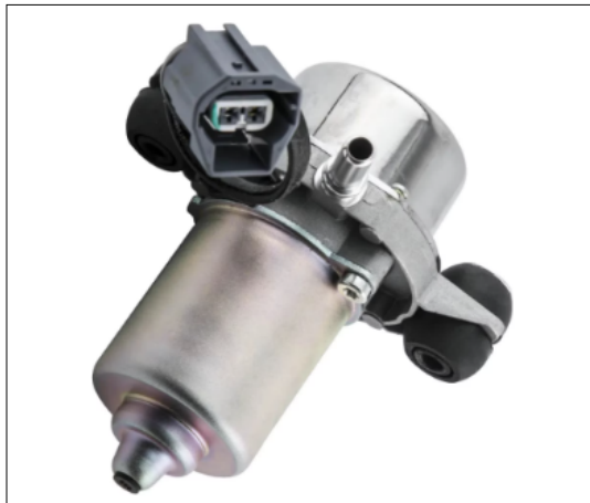
Fig. 7. Electric vacuum pump. [9]
