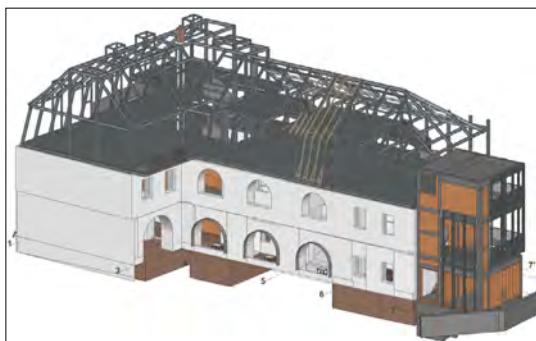
Fig. 2. Bolyai street 11 building 3D model.
