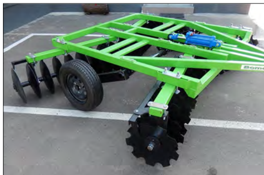
Fig. 1. Construction of the Bomet BTP 4×6 Disc Harrow.
