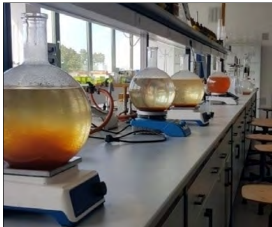
Fig. 1. Coagulation-flocculation chemical treatment.
