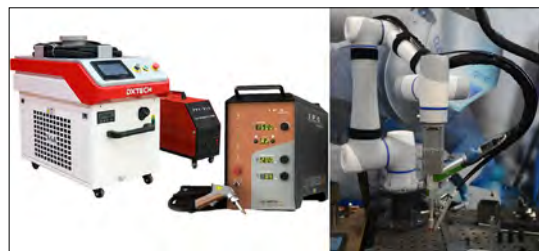
Fig. 3. Hand-held laser sources (left) and their integrated system with a cobot (right) [6]
