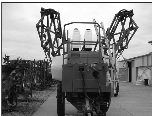
Fig. 4. Two 70 l tanks mounted on a RAU sprayer
