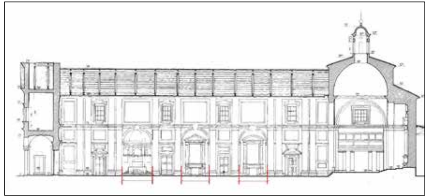
■ Fig. 11. Side elevation of the nave of St. Sebastian outside the walls, foregrounding the width of the chapels. © Augusto ROCA DE AMICIS
