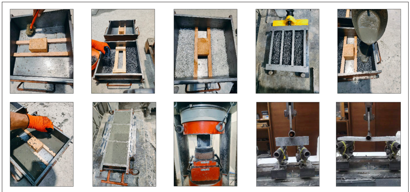
Fig. 2: Steps of pouring SIFCON concrete and test the different samples
