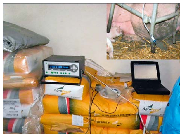
Figure 2: Measurement of the gas content of the barn air (Source: NARIC MGI)
