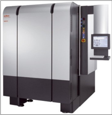
Fig. 3. INNOVA coating equipment.
