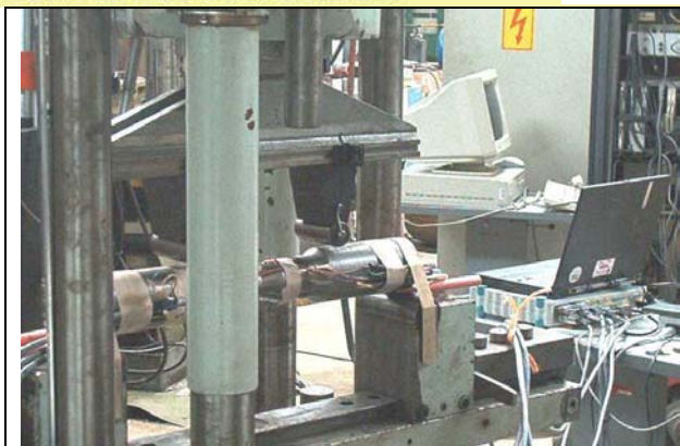
Fig.2: Static calibration of strain gauges on specimen to be tested
