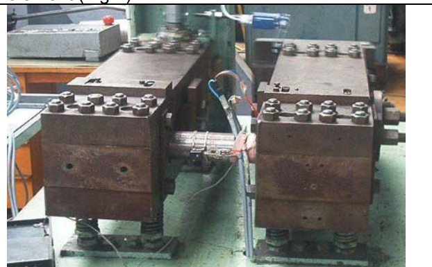
Fig.1: Machine resonance system with masses and tested specimen as a springy element
