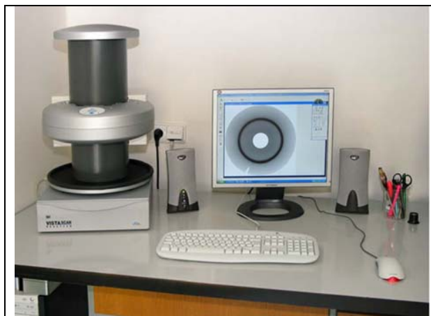
Fig. 4 Workplace for processing of imaging plate and for digital evaluating of diffraction patterns
