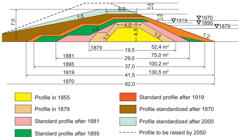
Fig. 3. Rise of the embankments (after VÁGÁS, I.)
