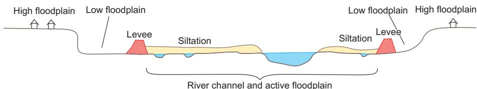
*Fig. 2. Rising of the flood control embankments since river regulation
