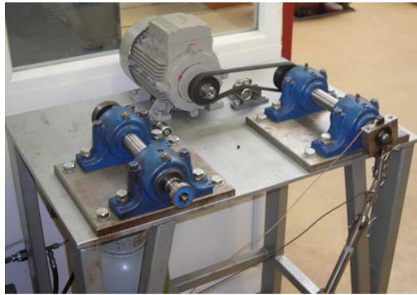
Figure 2. Bearing test rig in measurement position
