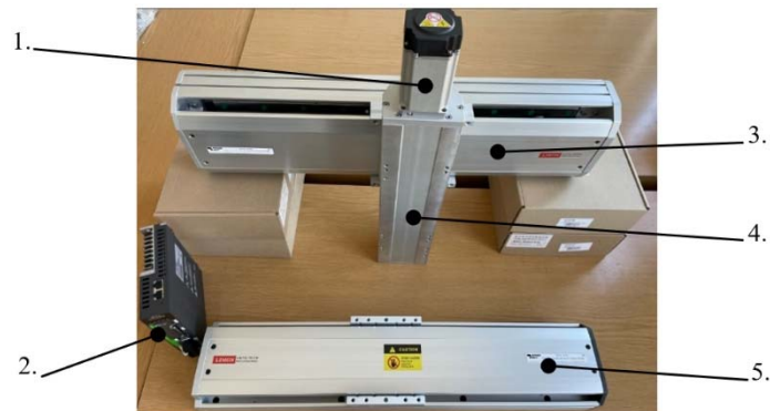
Figure 1. The linear units (3. – 5.) and one of the motors, motor drivers (1., 2.)
