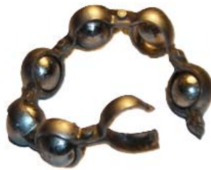
Figure 6. Failure of cage
