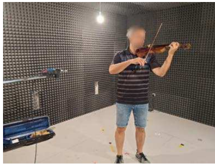
Figure 5. The measurement setup in semi-anechoic chamber
