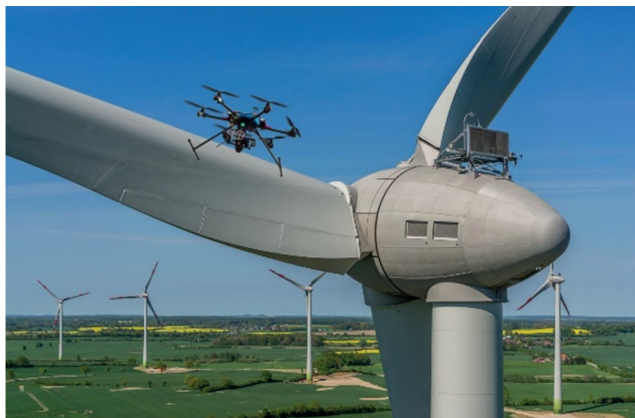
Figure 12. Inspection of wind turbines by X-ray technology [4]
