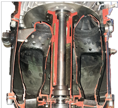
Figure 4. TKT-1 combustion chamber cross-section [the authors]
