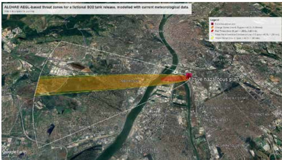
Figure 4 SO 2 tank release, which was modelled with current meteorological data
