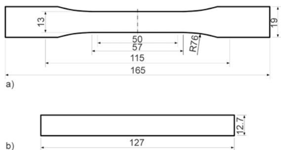
Figure 1. Specimen geometry, a) tensile and fatigue tests (ASTM D638 Type I), b) flexural tests (ASTM D790)
