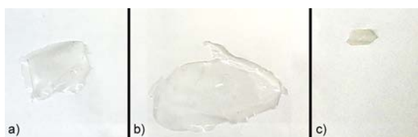
Figure 3. Dimension reversibility after 48 hr swelling in chloroform at room temperature, S3D3 (a), S3D5 (b), S5D3 (c). Original dimensions of all samples were similar before swelling.
