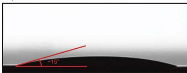
Figure 6. Illustrative images of the contact angle measurements for HDPE films with (a) water and (b) butyl acetate
