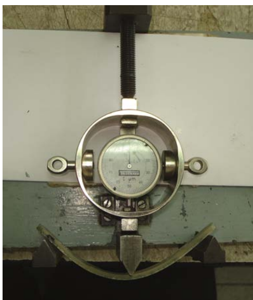
Figure 7. Snapshot showing the elastomer nature of composites with laboratory polymer matrix during bending tests
