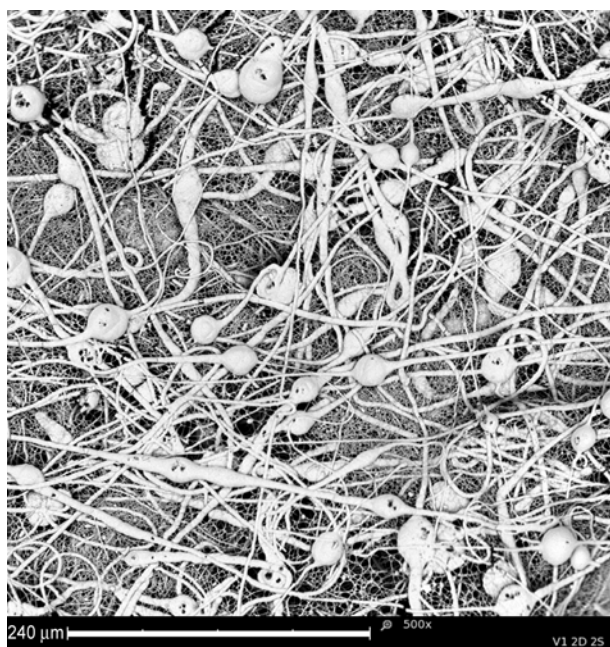
Figure 4. Scanning electron images of electrospun material: PCL fibers (from chloroform/ethanol 9:1 solution) wet electrospun into distilled water only. 2.5 mL of PCL polymer solution were used, which is five times more than for the production of other samples described here. The scale is 240 \mu\text{m} .
