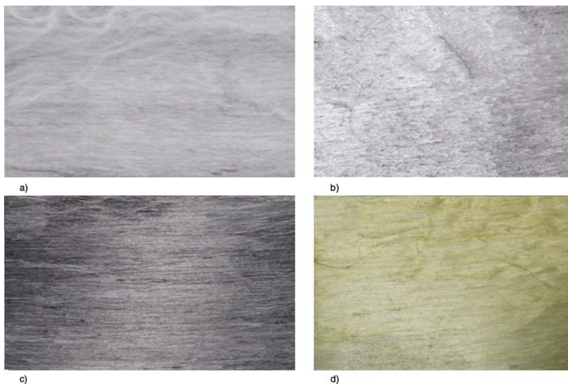
Figure 3. Photograph of (a) 100% PCL (b) 100% PVP (c) 50:50 PCL/PVP (d) drug loaded 50:50 PCL/PVP. The surface of C-spun fibers are rough and lack luster where as with corporation of PVP, the samples look lustrous due to the presence of homogeneity in diameter of the fibers.
