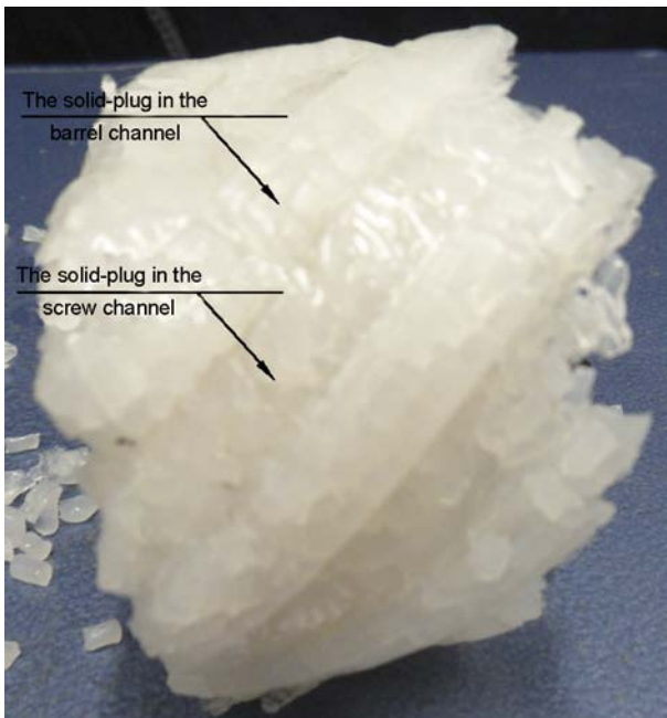
Figure 13. A whole solid-plug sample in a steady solids conveying process in the experimental extruder
