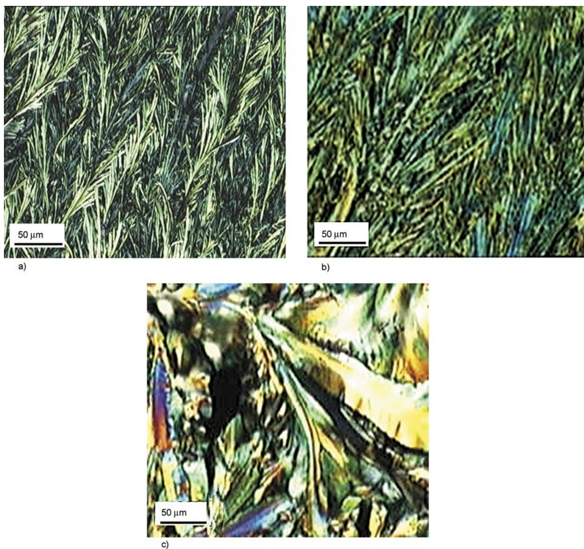
Figure 6. Room temperature morphology of thin sub. 3 and Polymer 1 layers (seen under crossed polarizes) after different thermal history: (a) – sub. 3 , cooling rate of 5 K/min; (b) – Polymer 1 , cooling rate of 5 K/min and (c) – Polymer 1 cooling rate of 1 K/min
