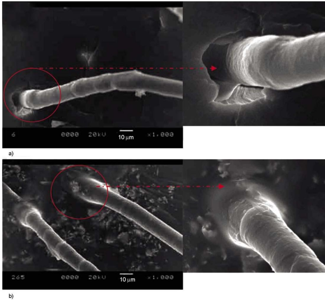
**Figure 9.** SEM photomicrographs of tensile fractured surfaces of 10 phr 6 mm short fiber loaded composite at the interface region (a) without any treatment (b) treated with 3 phr MA-g-PB
