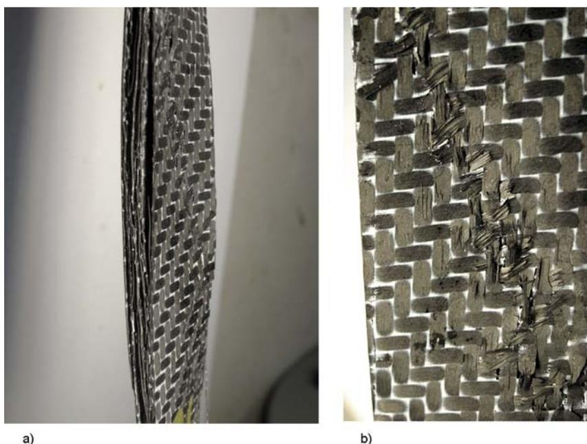
**Figure 4.** Typical tensile failure modes for the carbon/pCBT composites. (a) lateral view: delamination failure, (b) front view: shear breakage of bundle filaments.
