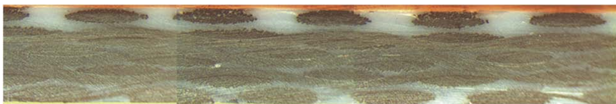
Figure 3. Light microscopic image of a srPET sample's cross section showing a good impregnation ( T_c 225°C/ t_h 6.5 min)
