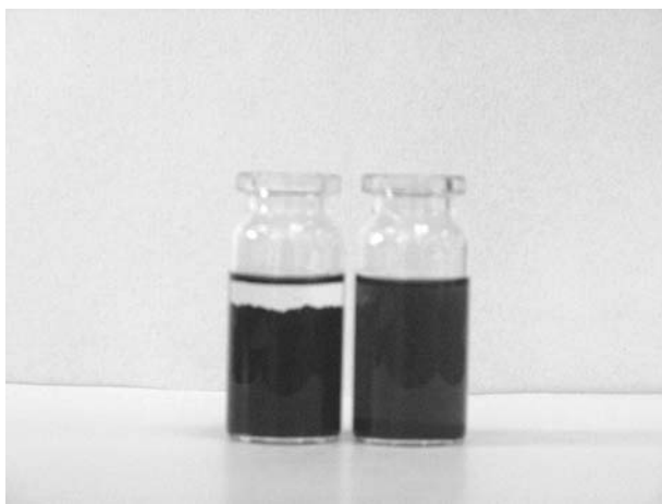
Figure 6. Photographs of the pristine MWCNTs (left) and the PVC-MWCNTs (right) dispersed in THF
