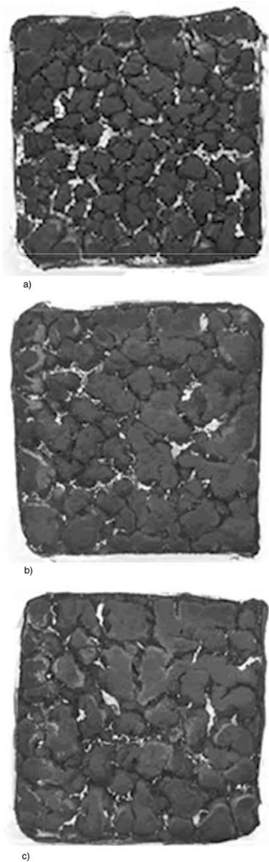
Figure 6. Pictures of the residues of nanocomposites after the cone experiment. a) PS/Cloisite 10A, b) PS/Cloisite 15A, c) PS/Nanofil 15 (pictures size of 75×75 mm)
