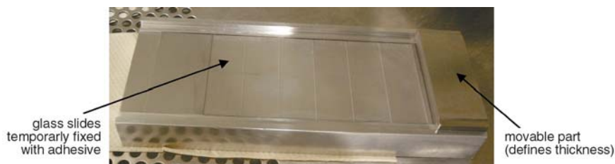
Figure 1. In-house developed setup for preparation of homogeneous PDMS coatings with defined thickness onto standard microscope slides
