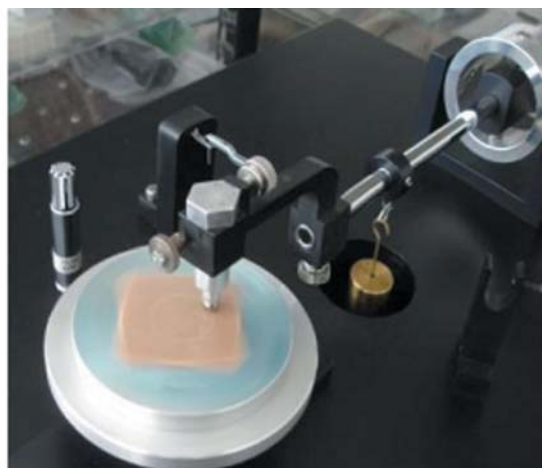
Figure 1. Schematic (left) of the pin-on-disk tribometer (right) illustrating the testing set-up for the friction and wear characterization of rubber sample (mounted on disk) against a counter-surface (pin/steel ball)
